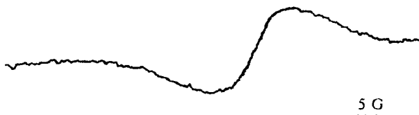
Fig. 3. ESR spectrum of the paramagnetic product of radical dehydrogenation of C_{60}H_{36} at 300 K.
